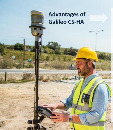
High Accuracy (CS-HA): receiver positioning accuracy with an **error below one decimetre**
