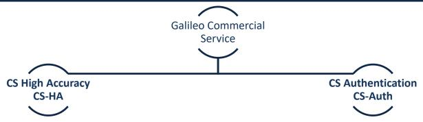
**CS-HA** - a controlled high accuracy service based on Precise Point Positioning (PPP) corrections transmitted in the E6 CS signal (E6-B, data component)
